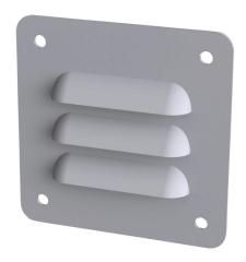
Saginaw louver vent, 3.25 x 3.25in (HxW), carbon steel, ANSI 61 gray, powder coat finish, 2.00 x 1.75in (HxW) cutout, for ventilation of metal enclosure. Mounting hardware included.
