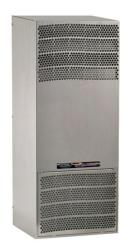
Saginaw Enviro-Therm air conditioner, 2550 BTU/H, R-134a, 460 VAC operating voltage, 316 stainless steel housing, side mount. For use with NEMA/UL Type 3R, 4, 4X & 12 enclosures.
