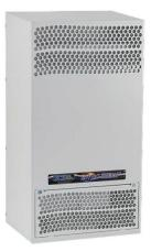
Saginaw Enviro-Therm air conditioner, 1000 BTU/H, R-134a, 230 VAC operating voltage, carbon steel housing, RAL 7035 light gray, side mount. For use with NEMA/UL Type 3R, 4 & 12 enclosures.
