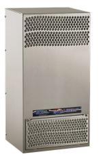
Saginaw Enviro-Therm air conditioner, 1000 BTU/H, R-134a, 230 VAC operating voltage, 304 stainless steel housing, side mount. For use with NEMA/UL Type 3R, 4, 4X & 12 enclosures.
