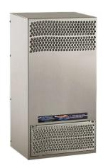
Saginaw Enviro-Therm air conditioner, 1000 BTU/H, R-134a, 230 VAC operating voltage, 316 stainless steel housing, side mount. For use with NEMA/UL Type 3R, 4, 4X & 12 enclosures.
