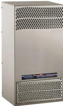
Saginaw Enviro-Therm air conditioner, 1000 BTU/H, R-134a, 115 VAC operating voltage, 316 stainless steel housing, side mount. For use with NEMA/UL Type 3R, 4, 4X & 12 enclosures.
