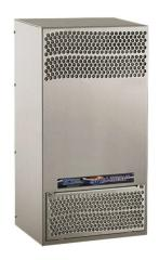
Saginaw Enviro-Therm air conditioner, 1000 BTU/H, R-134a, 115 VAC operating voltage, 316 stainless steel housing, side mount. For use with NEMA/UL Type 3R, 4, 4X & 12 enclosures.
