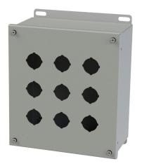
Saginaw pushbutton enclosure, 9 holes, 30mm, NEMA 4/12/13, 10 x 9 x 5in (HxWxD), wall mount, carbon steel, ANSI 61 gray, powder coat finish, screw cover.
