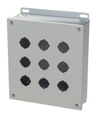
Saginaw pushbutton enclosure, 9 holes, 30mm, NEMA 4/4X/12/13, 10 x 9 x 3in (HxWxD), wall mount, 304 stainless steel, #4 brush finish, screw cover.
