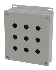
Saginaw pushbutton enclosure, 9 holes, 22mm, NEMA 4/12/13, 10 x 9 x 3in (HxWxD), wall mount, carbon steel, ANSI 61 gray, powder coat finish, screw cover.
