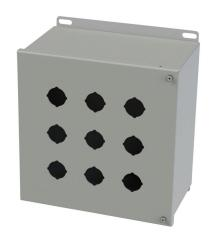
Saginaw pushbutton enclosure, 9 holes, 30mm, NEMA 4/12/13,  $10 \times 10 \times 6$ in (HxWxD), wall mount, carbon steel, ANSI 61 gray, powder coat finish, hinged screw cover.
