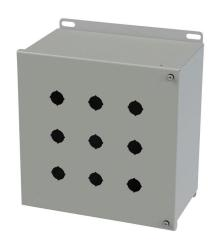
Saginaw pushbutton enclosure, 9 holes, 22mm, NEMA 4/12/13,  $10 \times 10 \times 6$ in (HxWxD), wall mount, carbon steel, ANSI 61 gray, powder coat finish, hinged screw cover.
