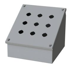
Saginaw pushbutton consolet, 9 holes, 22mm, NEMA 4/12/13, 9 x 9 x 8in (HxWxD), wall mount, carbon steel, ANSI 61 gray, powder coat finish, screw cover, purchase subpanel separately.
