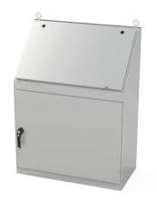
Saginaw operator console, NEMA 3R/12/13, 48 x 36 x 18in (HxWxD), freestanding, carbon steel, ANSI 61 gray, powder coat finish, single-door, 3-point keylocking/padlocking combo handle.
