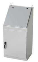
Saginaw operator console, NEMA 3R/12/13, 48 x 24 x 18in (HxWxD), freestanding, carbon steel, ANSI 61 gray, powder coat finish, single-door, 3-point keylocking/padlocking combo handle.
