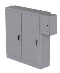
Saginaw enclosure, NEMA 3R/12/13, 90 x 78 x 18in (HxWxD), freestanding, carbon steel, ANSI 61 gray, powder coat finish, 2-door, 3-point padlocking handle, subpanel and external rotary disconnect enclosure included.
