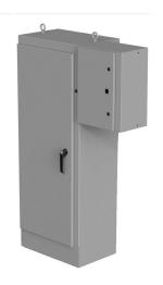
Saginaw enclosure, NEMA 3R/12/13, 90 x 40 x 18in (HxWxD), freestanding, carbon steel, ANSI 61 gray, powder coat finish, single-door, 3-point padlocking handle, external rotary disconnect enclosure included.
