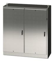
Saginaw disconnect enclosure, NEMA 3R/4/4X/12/13, right flange, 90 x 78 x 24in (HxWxD), freestanding, 304 stainless steel, #4 brush finish, 2-door, 3-point padlocking handle, powder coated subpanel included.
