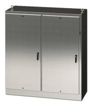
Saginaw disconnect enclosure, NEMA 3R/4/4X/12/13, right flange, 90 x 78 x 24in (HxWxD), freestanding, 316L stainless steel, #4 brush finish, 2-door, 3-point padlocking handle, powder coated subpanel included.
