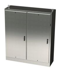
Saginaw disconnect enclosure, NEMA 3R/4/4X/12/13, right flange, 90 x 78 x 18in (HxWxD), freestanding, 304 stainless steel, #4 brush finish, 2-door, 3-point padlocking handle, powder coated subpanel included.
