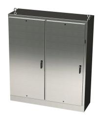
Saginaw disconnect enclosure, NEMA 3R/4/4X/12/13, right flange, 90 x 78 x 18in (HxWxD), freestanding, 316L stainless steel, #4 brush finish, 2-door, 3-point padlocking handle, powder coated subpanel included.
