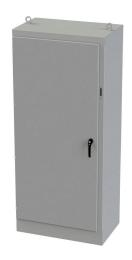
Saginaw disconnect enclosure, NEMA 3R/12/13, right flange,  $90 \times 40 \times 24$ in (HxWxD), freestanding, carbon steel, ANSI 61 gray, powder coat finish, single-door, 3-point padlocking handle, galvanized subpanel included.
