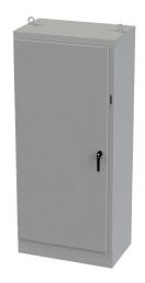
Saginaw disconnect enclosure, NEMA 3R/12/13, right flange,  $90 \times 40 \times 24$ in (HxWxD), freestanding, carbon steel, ANSI 61 gray, powder coat finish, single-door, 3-point padlocking handle, galvanized subpanel included.
