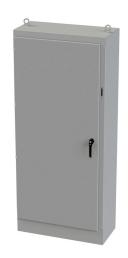
Saginaw disconnect enclosure, NEMA 3R/12/13, right flange,  $90 \times 40 \times 18$  in (HxWxD), freestanding, carbon steel, ANSI 61 gray, powder coat finish, single-door, 3-point padlocking handle, powder coated subpanel included.
