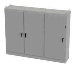
Saginaw disconnect enclosure, NEMA 3R/12/13, right flange, 90 x 118 x 24in (HxWxD), freestanding, carbon steel, ANSI 61 gray, powder coat finish, 3-door, 3-point padlocking handle, (2) powder coated subpanels included.
