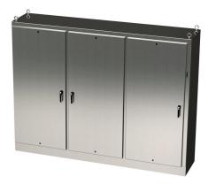
Saginaw disconnect enclosure, NEMA 3R/4/4X/12/13, right flange, 90 x 118 x 24in (HxWxD), freestanding, 316L stainless steel, #4 brush finish, 3-door, 3-point padlocking handle, (2) powder coated subpanels included.
