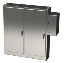
Saginaw enclosure, NEMA 3R/4/4X/12/13, 90 x 78 x 18in (HxWxD), freestanding, 304 stainless steel, #4 brush finish, 2-door, 3-point padlocking handle, external disconnect enclosure included.
