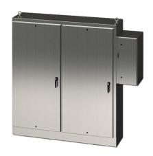
Saginaw enclosure, NEMA 3R/4/4X/12/13, 90 x 78 x 18in (HxWxD), freestanding, 316L stainless steel, #4 brush finish, 2-door, 3-point padlocking handle, external disconnect enclosure included.
