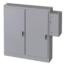
Saginaw enclosure, NEMA 3R/12/13, 90 x 78 x 18in (HxWxD), freestanding, carbon steel, ANSI 61 gray, powder coat finish, 2-door, 3-point padlocking handle, subpanel and external disconnect enclosure included.
