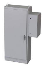
Saginaw enclosure, NEMA 3R/12/13, 90 x 40 x 18in (HxWxD), freestanding, carbon steel, ANSI 61 gray, powder coat finish, single-door, 3-point padlocking handle, external disconnect enclosure included.
