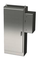
Saginaw enclosure, NEMA 3R/4/4X/12/13, 90 x 40 x 18in (HxWxD), freestanding, 304 stainless steel, #4 brush finish, single-door, 3-point padlocking handle, external disconnect enclosure included.
