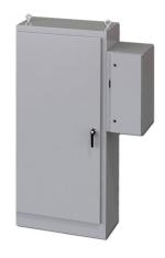
Saginaw enclosure, NEMA 3R/12/13, 90 x 40 x 18in (HxWxD), freestanding, carbon steel, ANSI 61 gray, powder coat finish, single-door, 3-point padlocking handle, subpanel and external disconnect enclosure included.
