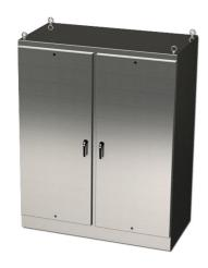
Saginaw Enviroline series enclosure, NEMA 3R/4/4X/12/13, 90 x 72 x 36in (HxWxD), freestanding, 316L stainless steel, #4 brush finish, 2-door, 3-point keylocking/padlocking combo handle.
