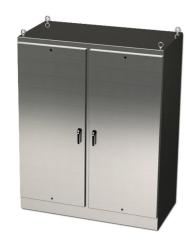
Saginaw Enviroline series enclosure, NEMA 3R/4/4X/12/13, 90 x 72 x 24in (HxWxD), freestanding, 316L stainless steel, #4 brush finish, 2-door, 3-point keylocking/padlocking combo handle.
