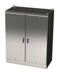
Saginaw Enviroline series enclosure, NEMA 3R/4/4X/12/13, 90 x 72 x 20in (HxWxD), freestanding, 304 stainless steel, #4 brush finish, 2-door, 3-point keylocking/padlocking combo handle.
