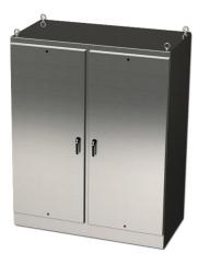
Saginaw Enviroline series enclosure, NEMA 3R/4/4X/12/13, 90 x 48 x 20in (HxWxD), freestanding, 316L stainless steel, #4 brush finish, 2-door, 3-point keylocking/padlocking combo handle.
