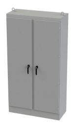
Saginaw Enviroline series enclosure, NEMA 3R/4/12/13, 90 x 48 x 20in (HxWxD), freestanding, carbon steel, ANSI 61 gray, powder coat finish, 2-door, 3-point keylocking/padlocking combo handle.
