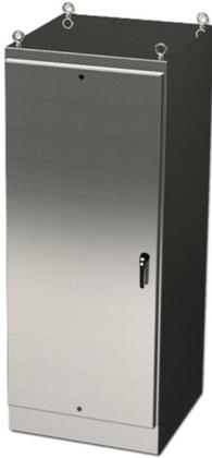
Saginaw Enviroline series enclosure, NEMA 3R/4/4X/12/13, 90 x 36 x 24in (HxWxD), freestanding, 304 stainless steel, #4 brush finish, single-door, 3-point keylocking/padlocking combo handle.
