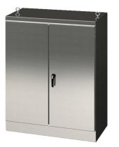
Saginaw enclosure, NEMA 3R/12/13, 90 x 72 x 36in (HxWxD), freestanding, 304 stainless steel, #4 brush finish, double-door, 3-point keylocking/padlocking combo handle.
