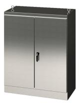
Saginaw enclosure, NEMA 3R/12/13, 90 x 72 x 24in (HxWxD), freestanding, 304 stainless steel, #4 brush finish, double-door, 3-point keylocking/padlocking combo handle.
