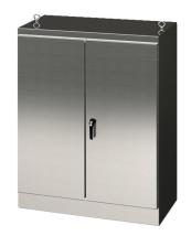
Saginaw enclosure, NEMA 3R/12/13, 90 x 72 x 20in (HxWxD), freestanding, 304 stainless steel, #4 brush finish, double-door, 3-point keylocking/padlocking combo handle.
