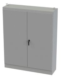
Saginaw enclosure, NEMA 3R/12/13, 90 x 72 x 20in (HxWxD), freestanding, carbon steel, ANSI 61 gray, powder coat finish, double-door, 3-point keylocking/padlocking combo handle.
