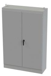
Saginaw enclosure, NEMA 3R/12/13, 90 x 60 x 20in (HxWxD), freestanding, carbon steel, ANSI 61 gray, powder coat finish, double-door, 3-point keylocking/padlocking combo handle.
