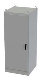
Saginaw enclosure, NEMA 3R/12/13, 90 x 36 x 36in (HxWxD), freestanding, dual access, carbon steel, ANSI 61 gray, powder coat finish, single-door, 3-point keylocking/padlocking combo handle.
