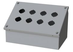
Saginaw pushbutton consolet, 8 holes, 30mm, NEMA 4/12/13, 7 x 11 x 7in (HxWxD), wall mount, carbon steel, ANSI 61 gray, powder coat finish, screw cover, purchase subpanel separately.
