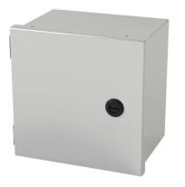
Saginaw enclosure, NEMA 1, 8 x 8 x 6in (HxWxD), wall mount, carbon steel, ANSI 61 gray, powder coat finish, single-door, 1/4-turn semi-flush latch.
