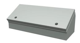
Saginaw operator consolet, NEMA 3R/4/12/13, 8 x 20 x 7in (HxWxD), desktop or pedestal mount, carbon steel, ANSI 61 gray, powder coat finish, single-door, 1/4-turn semi-flush latch.
