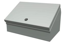
Saginaw operator consolet, NEMA 3R/4/12/13, 8 x 12 x 7in (HxWxD), desktop or pedestal mount, carbon steel, ANSI 61 gray, powder coat finish, single-door, 1/4-turn semi-flush latch.
