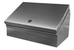
Saginaw operator consolet, NEMA 3R/4/4X/12/13, 8 x 12 x 7in (HxWxD), desktop or pedestal mount, 304 stainless steel, #4 brush finish, single-door, 1/4-turn semi-flush latch.
