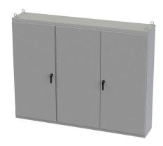
Saginaw enclosure, NEMA 3R/12/13, 86 x 112 x 20in (HxWxD), freestanding, carbon steel, ANSI 61 gray, powder coat finish, 3-door, 3-point padlocking handle.
