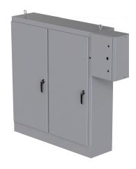
Saginaw enclosure, NEMA 3R/12/13, 84 x 78 x 18in (HxWxD), freestanding, carbon steel, ANSI 61 gray, powder coat finish, 2-door, 3-point padlocking handle, external rotary disconnect enclosure included.
