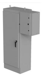
Saginaw enclosure, NEMA 3R/12/13, 84 x 40 x 18in (HxWxD), freestanding, carbon steel, ANSI 61 gray, powder coat finish, single-door, 3-point padlocking handle, external rotary disconnect enclosure included.
